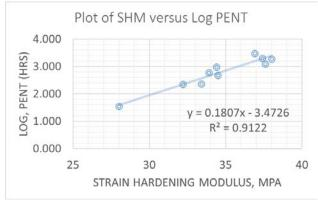
Figure 3. Plot of the log PENT values against the strain hardening modulus from Reference 14
