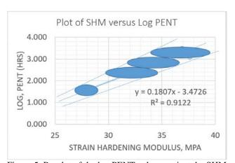
Figure 5. Re-plot of the log PENT values against the SHM for Figure 3 of this paper including superposition of ovals on top of some previous data points to illustrate error bars equal to 15% of the SHM measured value.
