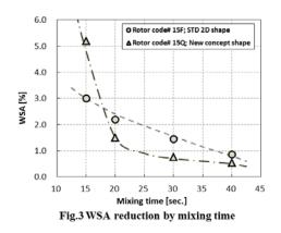
Until 15 seconds of mixing time, the 15F rotor profile provided better homogeneity performance than the 15Q rotor profile. After 20 seconds of mixing time, the 15Q rotor profile brought about better mixing performance than 15F rotor profile. The mixing performance features of respective rotor profiles are summarized in Table 2, below.
