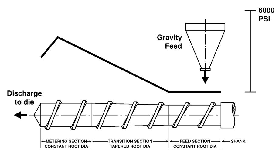
SSE are high pressure machines used mainly for pumping
