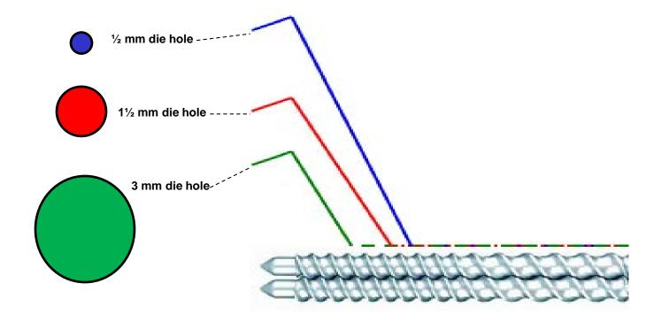
Thermo-mechanical devulcanization process with Supercritical CO<sub>2</sub> Process invented by Dr. C. Tsonganakis @ Univ. Waterloo
