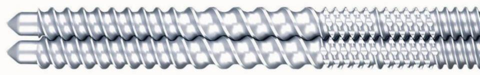
**Close meshing elements = more viscous heating**
