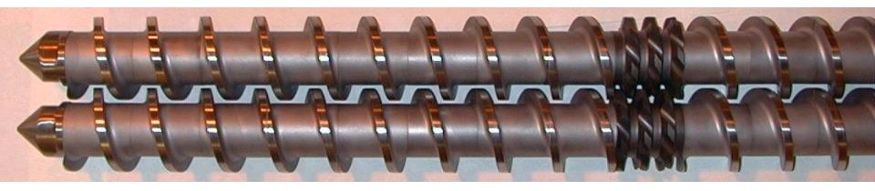
**Open meshing elements = better heat transfer/cooling**
