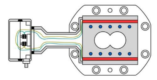
Internal cartridge heaters for electric heating
