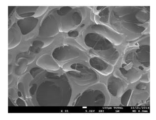
Figure 5. SEM image of conventional PP processed with 0.6mL/min CO<sub>2</sub> at 130 bar die pressure
