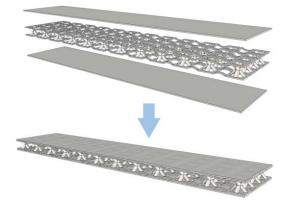
Figure 5. Plastic sandwich panel with pyramidal kagome core
