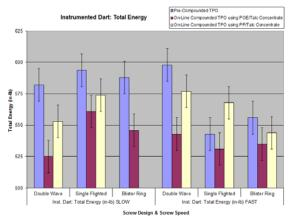
Figure 9: TPO Sheet - Instrumented Dart Impact.
