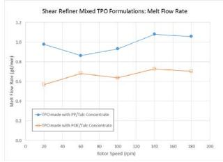
Figure 3: Shear Refiner Mixed TPO: Melt Flow Rate.
