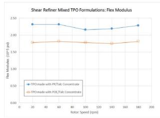
Figure 4: Shear Refiner Mixed TPO: Flex Modulus.
