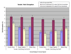
Figure 12: TPO Sheet – Tensile Elongation at Yield.
