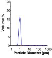
Figure 2. Particle size distribution of the polyolefin dispersion.
