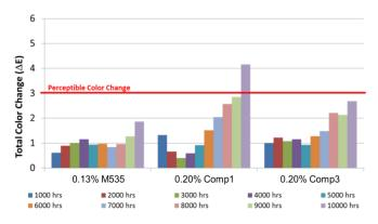
Figure 3 | Total color change in natural HDPE after 10k hours G155 weathering. Samples contain CYANOX<sup>®</sup> 2777 antioxidant.
