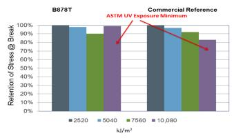
Figure 7 | TPO roofing sheet – retention of stress at break after 10,080  $kJ/(m^2 \cdot nm)$  radiant energy in an ASTM D6878 weatherometer
