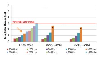
Figure 4 | Total color change in green HDPE after 10k hours G155 weathering. The (\*) denotes surface crazing.
