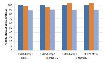
Figure 1 | Tensile data comparing CYASORB CYNERGY SOLUTIONS<sup>®</sup> M535 stabilizer to popular competitive stabilizers in HDPE with 1% white pigment masterbatch and CYANOX<sup>®</sup> 2777 antioxidant in ASTM G155 Cycle 1 Weathering
