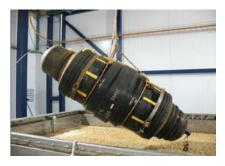
Figure 12. 630SDR17 Gas Pipe and Electrofusion Coupler During Hydrostatic Pressure Testing
