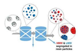
Figure 1. Staged-Reactor Bimodal HDPE Polymerization Process
