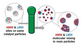
Figure 2. Single-Reactor PRODIGY BMC-200 Polymerization Process
