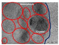
Figure 8. TEM image of Solid MAO-1(×500,000). \*Deep blue line shows a border of Solid MAO particle and a supporting film for TEM measurement.
