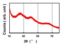
Figure 9. XRD measurement of Solid MAO.
