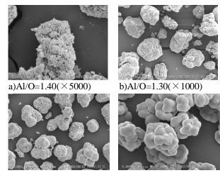
c)Al/O=1.25( $\times$ 1000) d)Al/O=1.20( $\times$ 5000) Figure 2. SEM images of Solid MAOs prepared by using various MAO solutions with different Al/O molar ratios.
