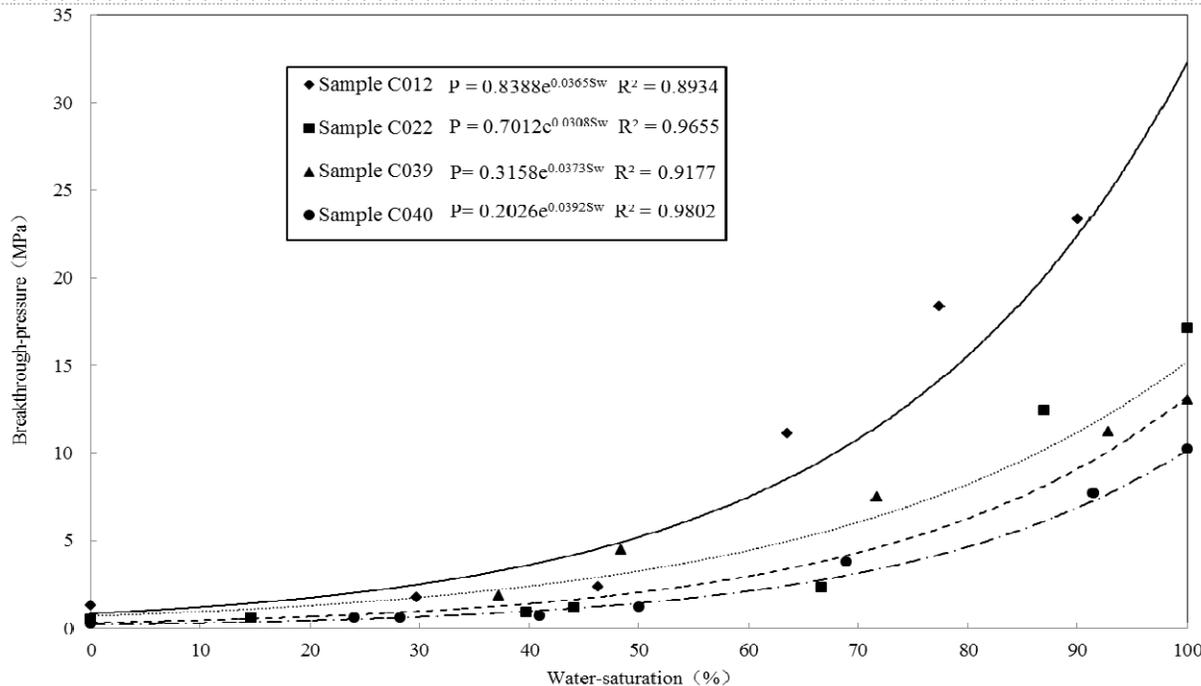
Fig.9 Comparison of the breakthrough pressure curves of the four samples (P: breakthrough pressure; Sw: water saturation).
