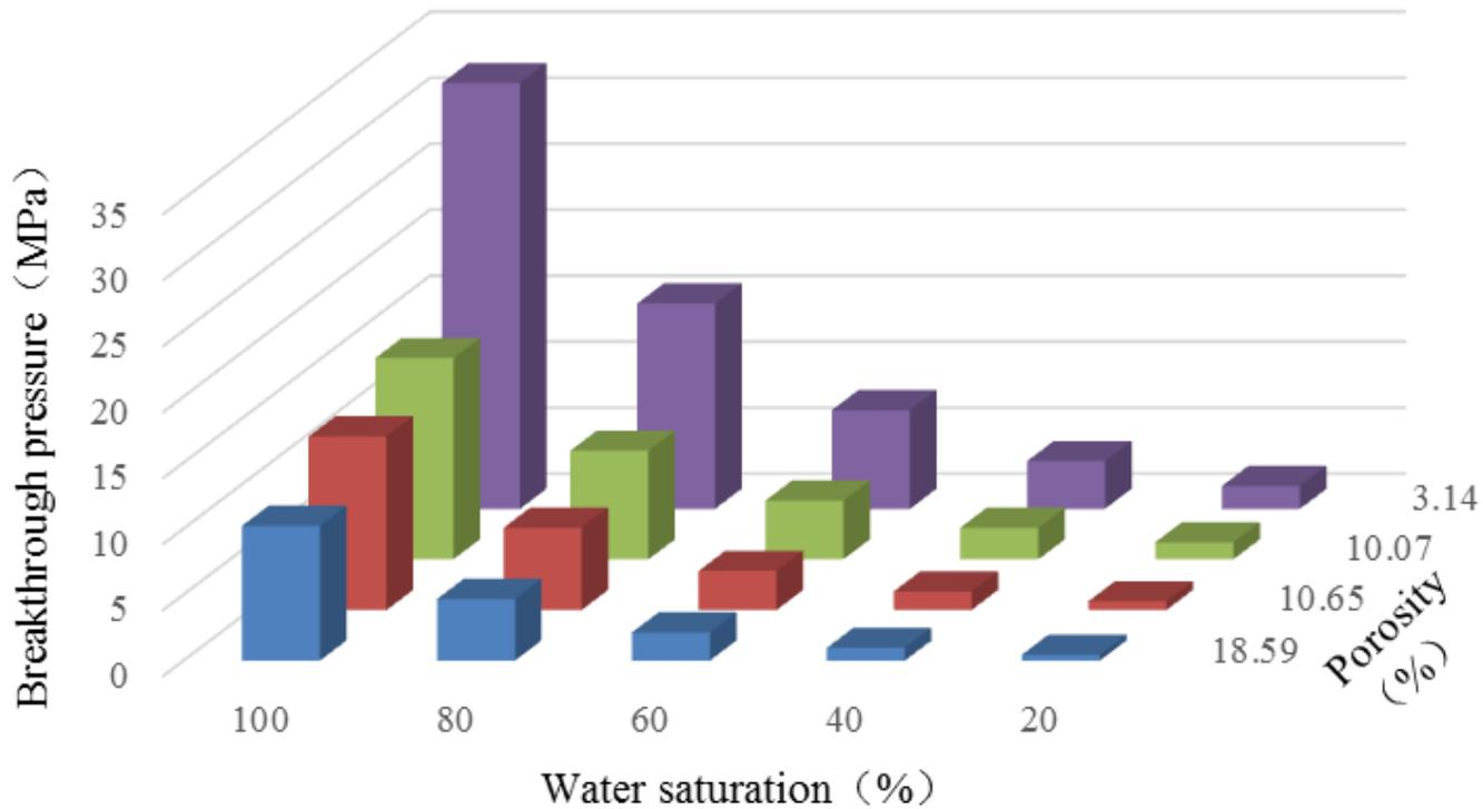
Fig.9 Graph of breakthrough pressure versus porosity versus water saturation for the four samples.
