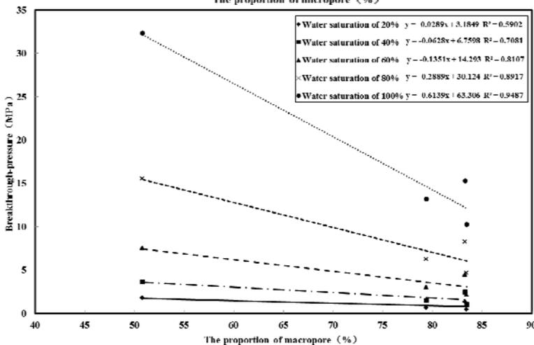
Fig.10 Relationships between proportion of each scale of micropores and breakthrough pressure (P: breakthrough pressure; r: ratio of the micropores).
