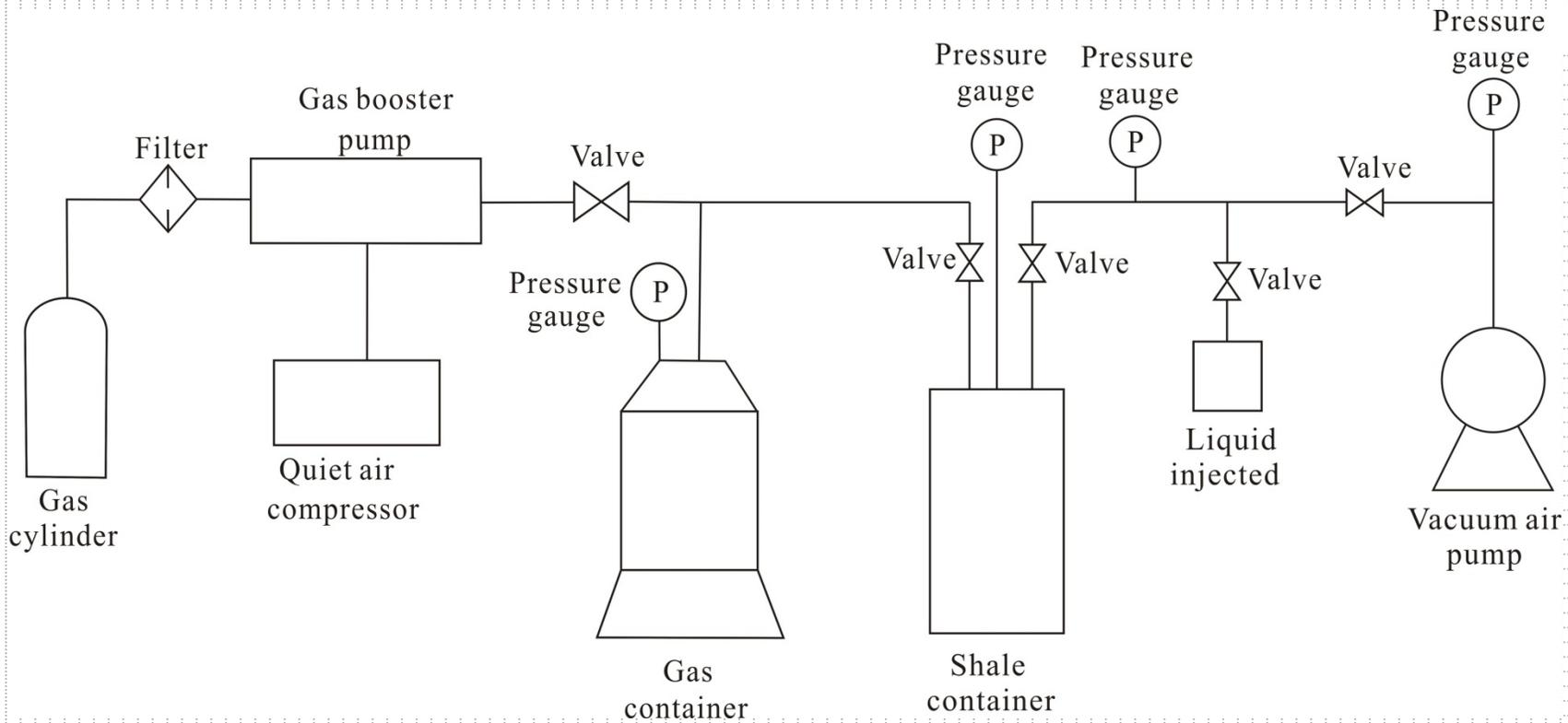
Fig.6 Schematic diagram of the water saturation experimental apparatus.
