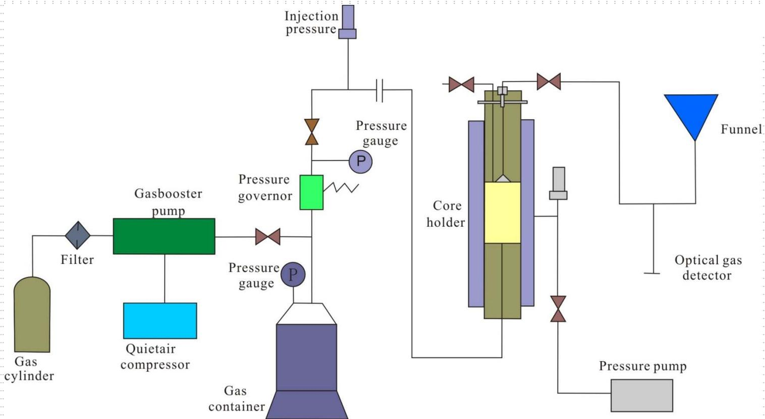
Fig.7 Schematic diagram of the breakthrough pressure detection apparatus.
