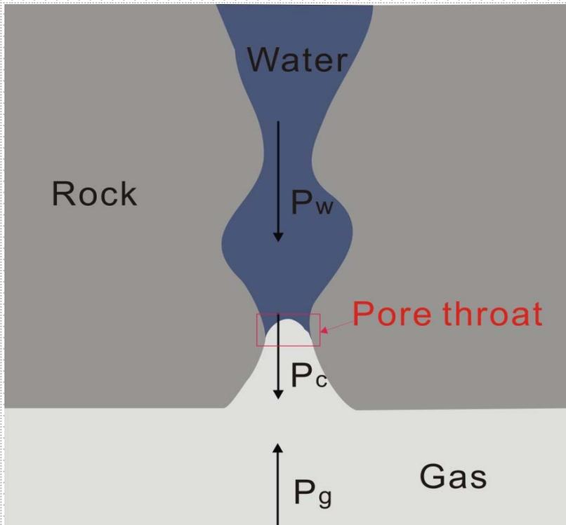
Fig.4 presents gas breakthrough mechanism in a pore throat. Capillary pressure ( $P_c$ ) in the low porous media in pore scale can be described by the Laplace equation:
