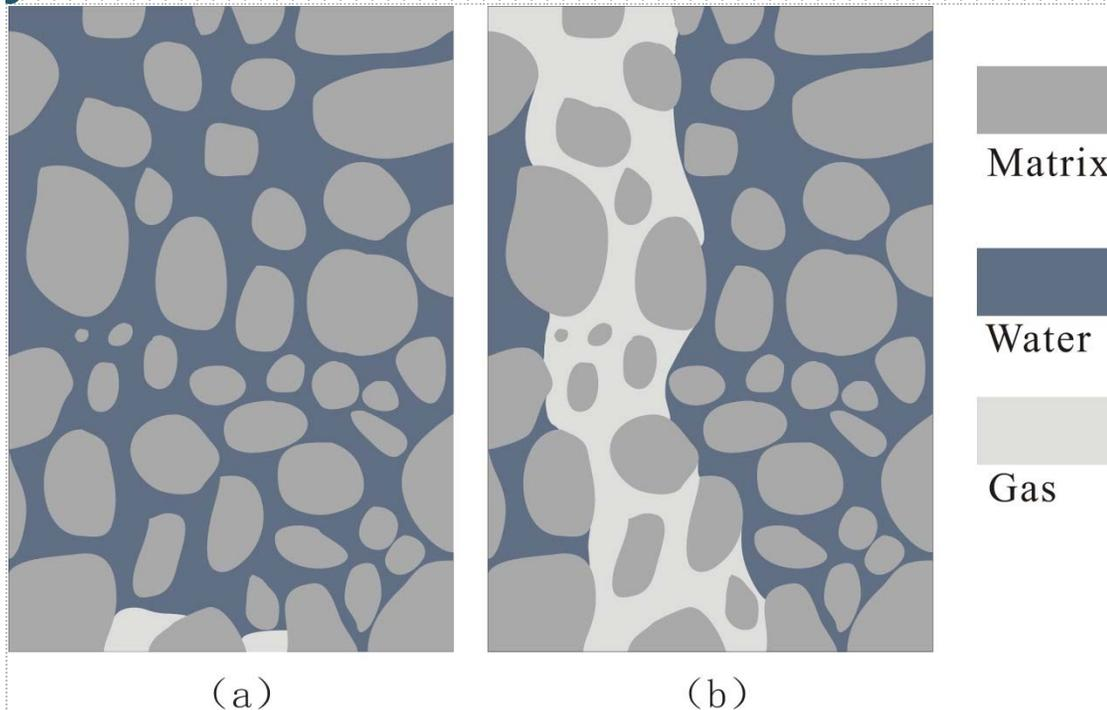
Fig.3 Two key points in process of gas flow in water-saturated rock: (a)  $P_c=P_{c,e}$ , gas started to permeate into the rock, and (b)  $P_c=P_{c,b}$ , gas flow pass the rock and gas leak is observed from the outlet of the rock
