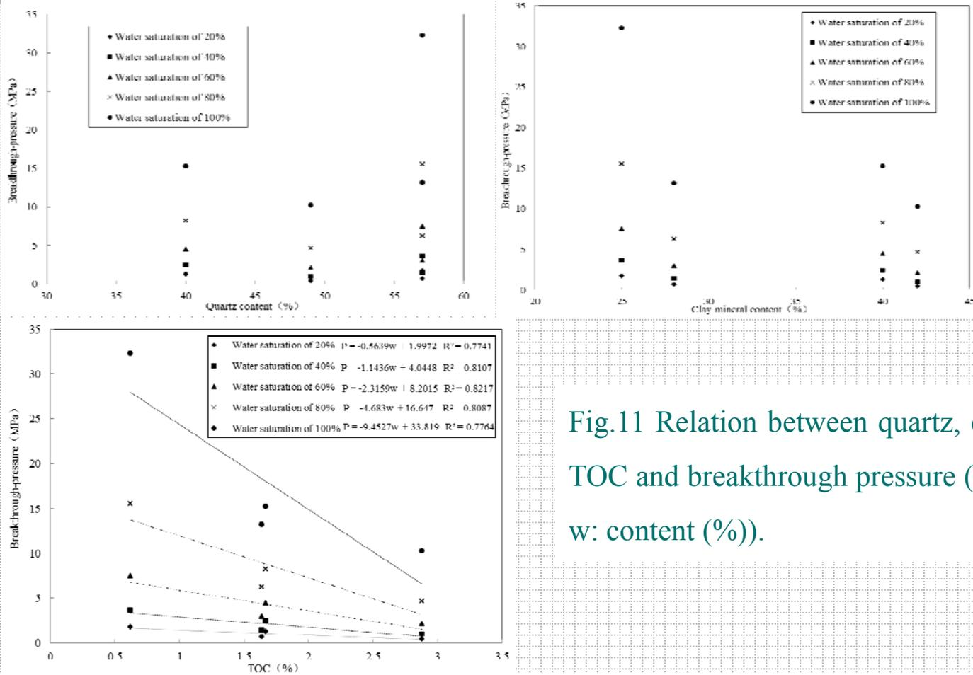
Fig.11 Relation between quartz, clay mineral content and TOC and breakthrough pressure (P: breakthrough pressure; w: content (%)).
