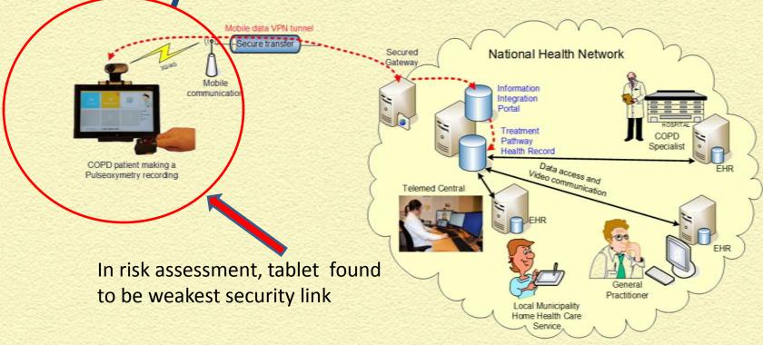
Solution: uses VPN SSL, web based secure connection (https); tablet functionality is locked down to only telehealth application use; user access security software on tablet; all data is encrypted at rest on tablet and in transmission to Health Network; de-identified data is transmitted from the tablet; two factor authentication methods are used; not using all of Continua guidelines
