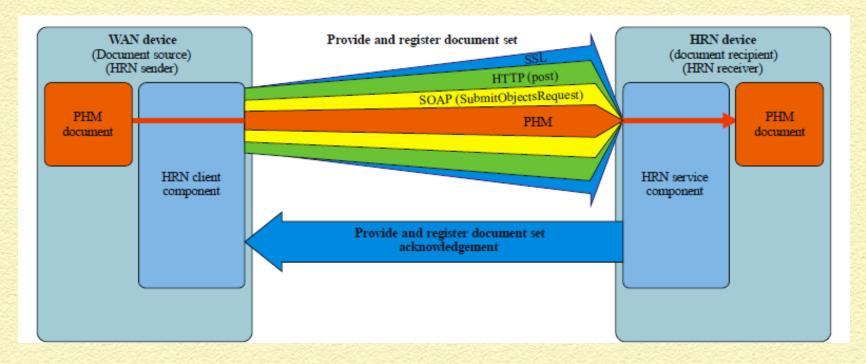
Uses VPN SSL, web based secure connection, which is administered at OSI layers 4.5, versus VPN IP Sec, which is administered at OSI layer 3
