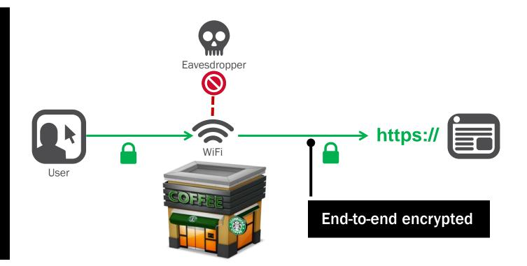
Important... passive SSL inspection (IPS/WAF/NGFW/...) require RSA-style session establishment because they work by doing a man-in-the-middle using the Server's private key. (This includes passive span-mode and bridge-mode devices.) With PFS only SSL termination /re-encryption will
