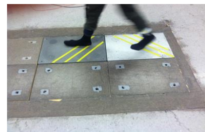
Figure 1: Exemplar subject stepping on each individual force platform while wearing the insoles.
