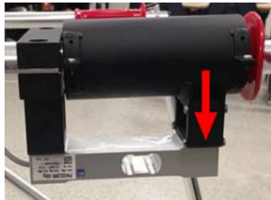
Figure 1: Photo of InvisiForce . The red arrow indicates location of vertical force applied by the surrogate handle on the load cell cantilever.
